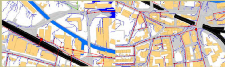
Flow pathways routed into canal
