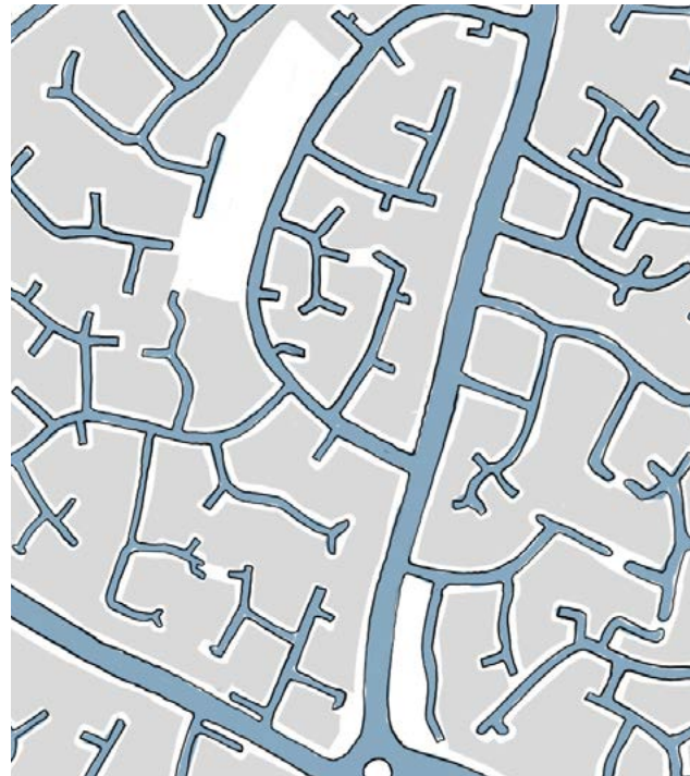
6. Connected Street Networks: A connected network of streets reduces walking distances.
