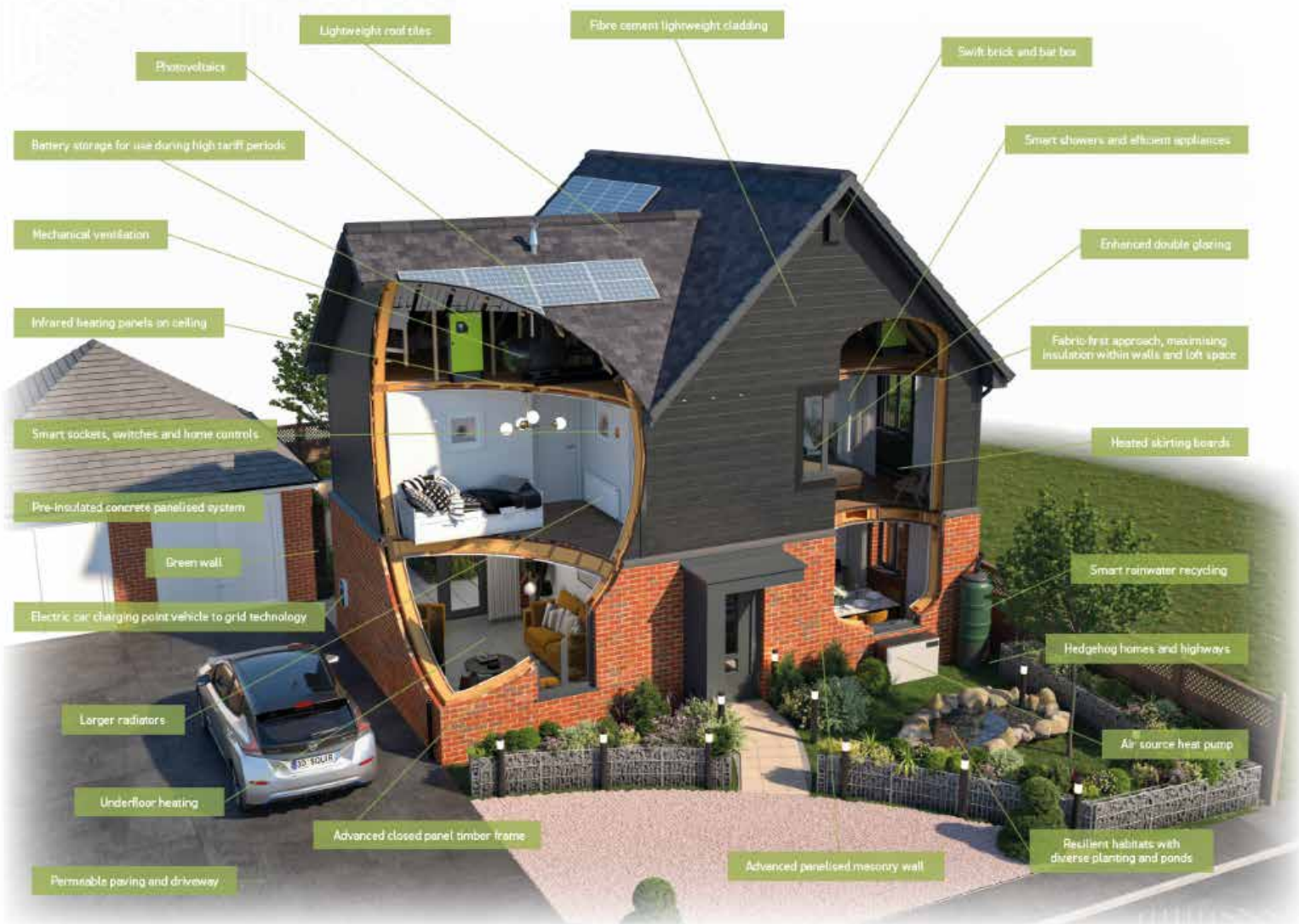
Typical David Wilson Home built to Future Homes Standard
