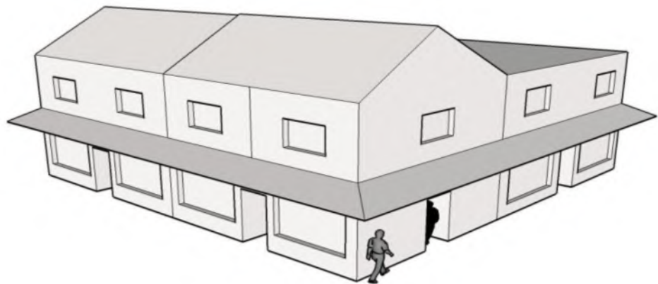
Canopies and recessed doorways can provide hiding places.
